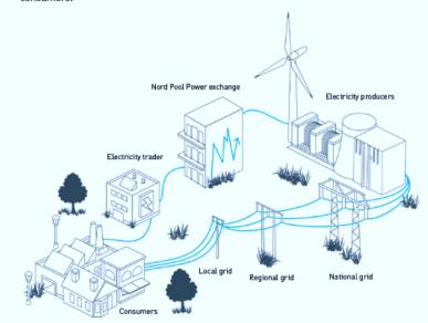
The diagram above shows the route of electricity from the producer (power station) via the national grid, regional network, local network and finally to the electricity consumer. The producers sell their electricity on the Nord Pool power exchange or to electricity suppliers. Suppliers sell the electricity on to the consumer.
